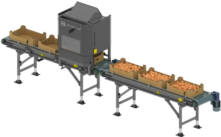
ANS with a conveyor belt for buffering crates or cartons
